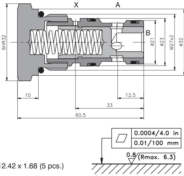
**TV2-102/M Meter-in compensator**
